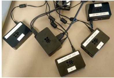
Figure 4.5: A network of 5 Raspberry Pi's interacting according to the ratio consensus protocol with the interaction network being the undirected network of Fig. 4.3. The communication between a device with its neighbor is through wifi.
