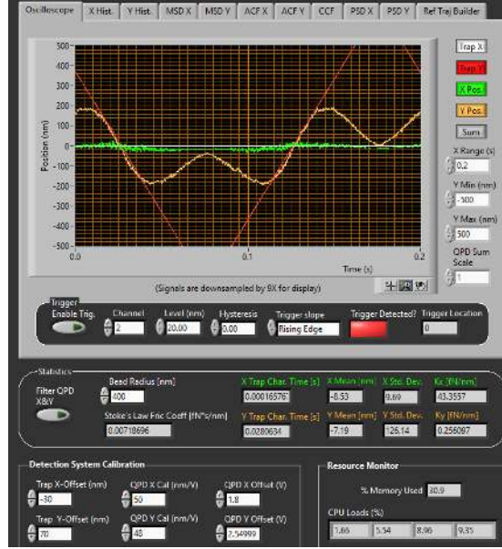
Figure 3.15: Example Oscilloscope Readout During Alignment
