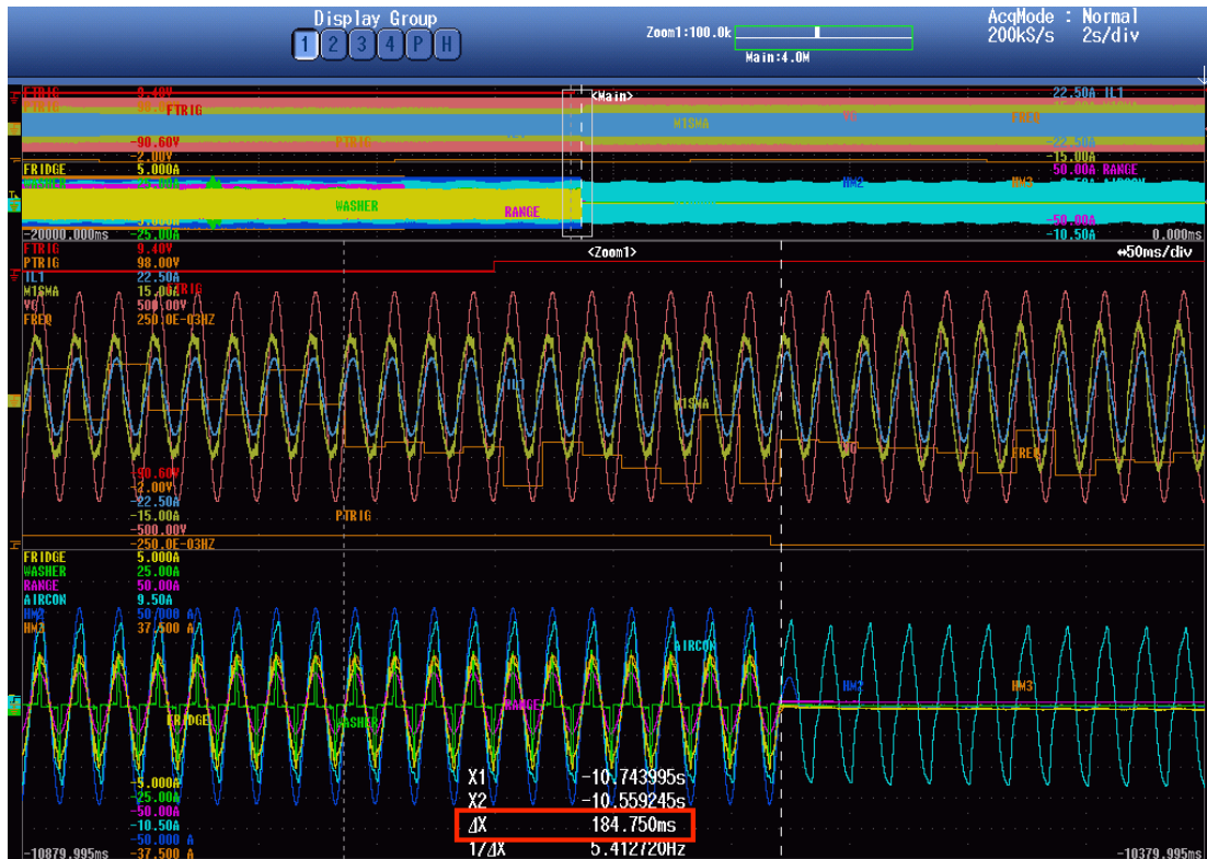
Figure 4.12: Trial #4 NLG dispatch results: Instantaneous waveforms (top) NLU1 inverter current (“IL1”), NLU2 inverter current (“M1SMA”), grid voltage (“VG”) and approximate grid frequency (“FREQ”). “FTRIG” goes from low to high when the local inverter controller detects the frequency event. “PTRIG” goes from high to low when the local inverter controller receives its dispatch set point from the NLGC. (bottom) Four NLU1 constituent load currents (“FRIDGE”, “WASHER”, “RANGE”, and “AIRCON”), the total load current of NLU1 (“HM3”), and the total load current of NLU2 (“HM2”).
