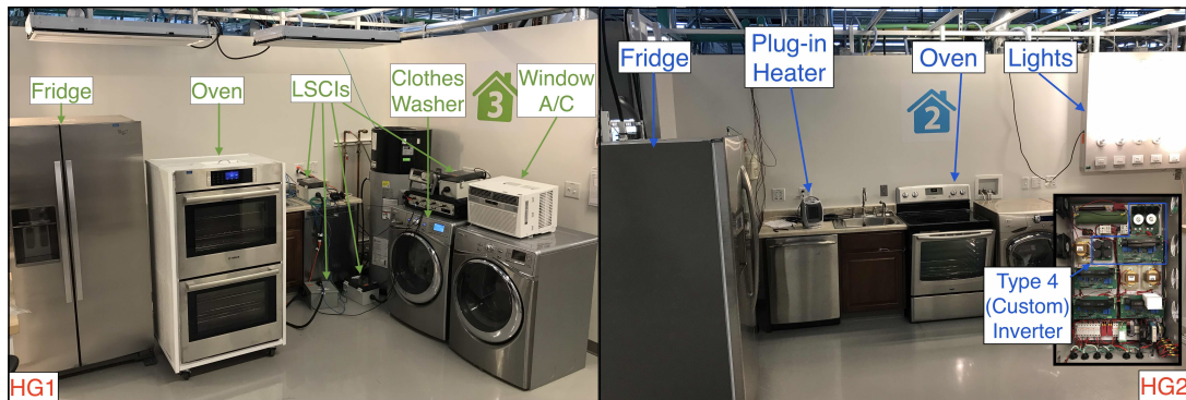
Figure 4.6: Photos of the two lab homes (HG1 and HG2) with residential appliance loads controlled denoted. One Type 4 (custom) inverter (pictured at right inset) is used with each HG.
